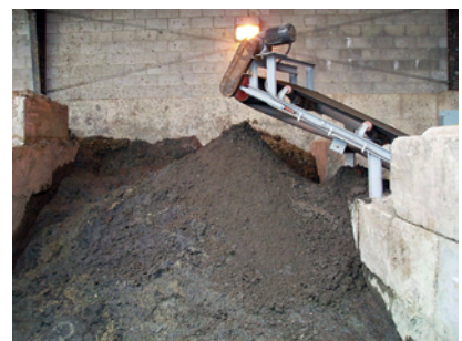
Dewatered Hydro Vac Mud
